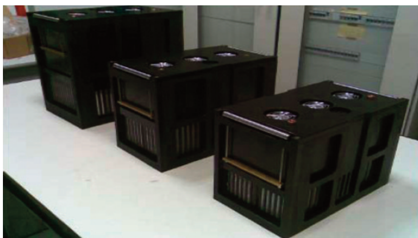
“Smart” 12 V Li-ion battery modules of 30/60/100 Ah
