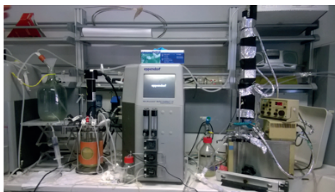
Experimental equipment for "fed-batch" fermentation with ethanol gas stripping
