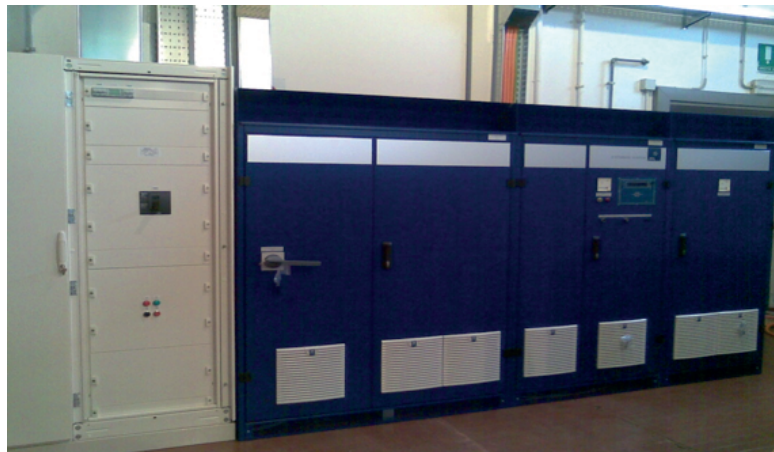
AVL 0-800 V Cyclator, I max ; 600 A, under both charge and discharge conditions
