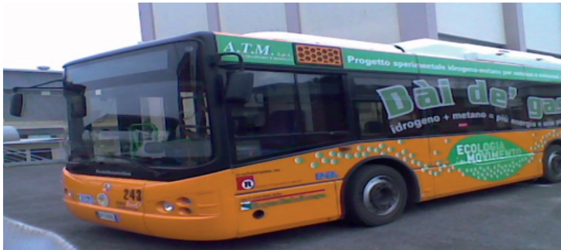
Bus 12 mt. powered with a mixture having a 15% content of Hydrogen, in Casaccia
