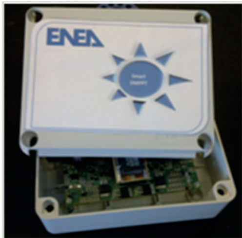
DMPPT converter tailored to PV systems
