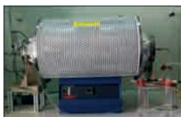
Tubular furnaces for the thermal treatment in flow of the PV modules
