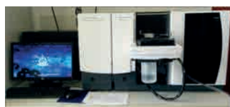
AA spectrophotometer for metals analysis in ashes, organic residues and gaseous emissions deriving from thermal treatment
