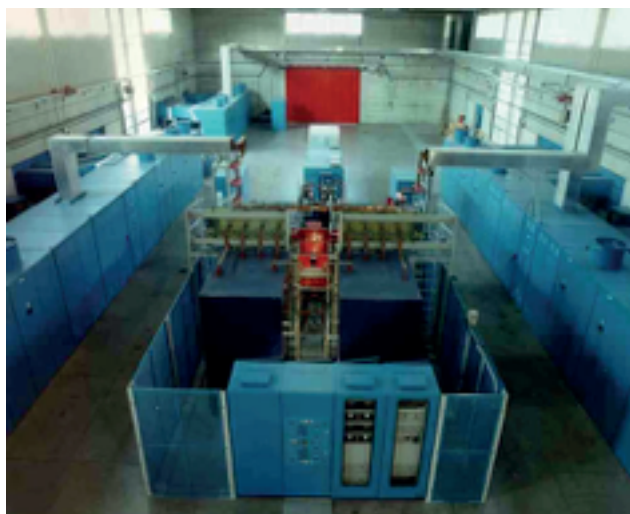
2016 - Tests to verify the Ecodesign transformer according to the EU Regulation 548/2014, requested by IMEFY S.p.A.
