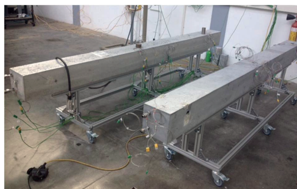
Concrete thermal energy storage modules
