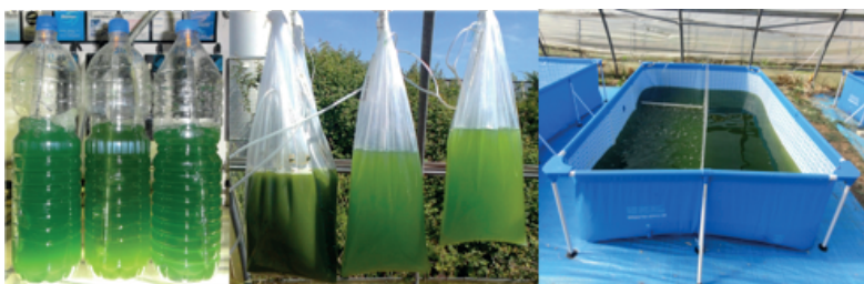
Microalgal cultures in low-cost containers. From left: 2 L mineral water bottles, 20 L polyethylene photobioreactors, 1,500 L plastic sheet tank equipped with an air lift aerator / agitator with inclined plane
