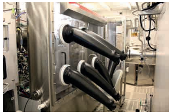
Deposition system for thin films for OLEDs, integrated with a glove box to reduce the Oxygen and moisture levels (O2 and H2O < 1 ppm).
