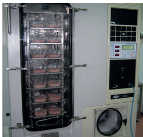
2- VIRTIS Genesis 35 ES freeze dryer at pilot scale, at the CR Trisaia (MT)
