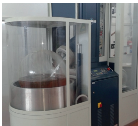
1- STRIKE 5000 vacuum evaporation plant
