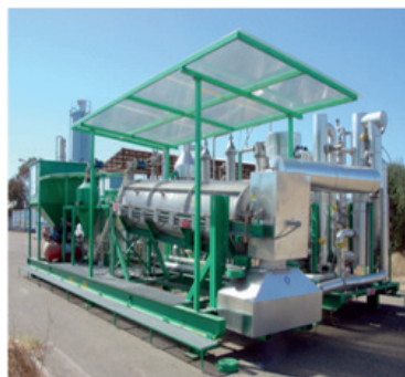
Rotating drum gasifier
