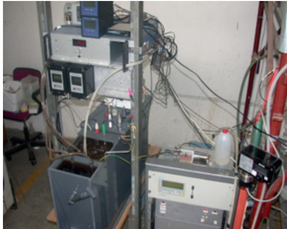
Microbial fuel cell membraneless with management and control device (Patent B02006A879)
