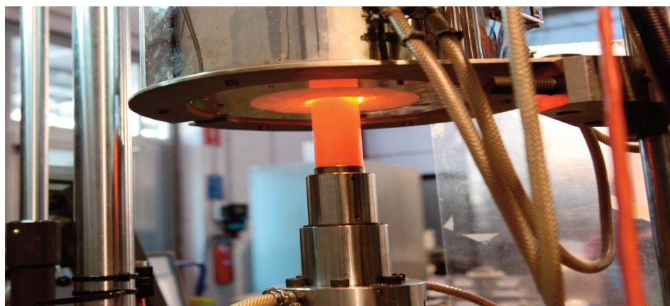
MTS testing machine, equipped with furnace, to perform bending test up to 1500 °C
