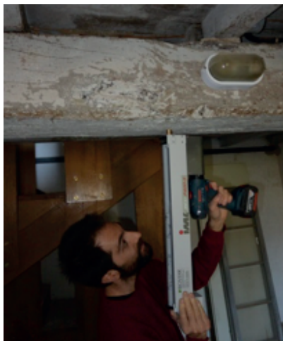
Fig. 1 - Montorio Castle: Resistographic test
