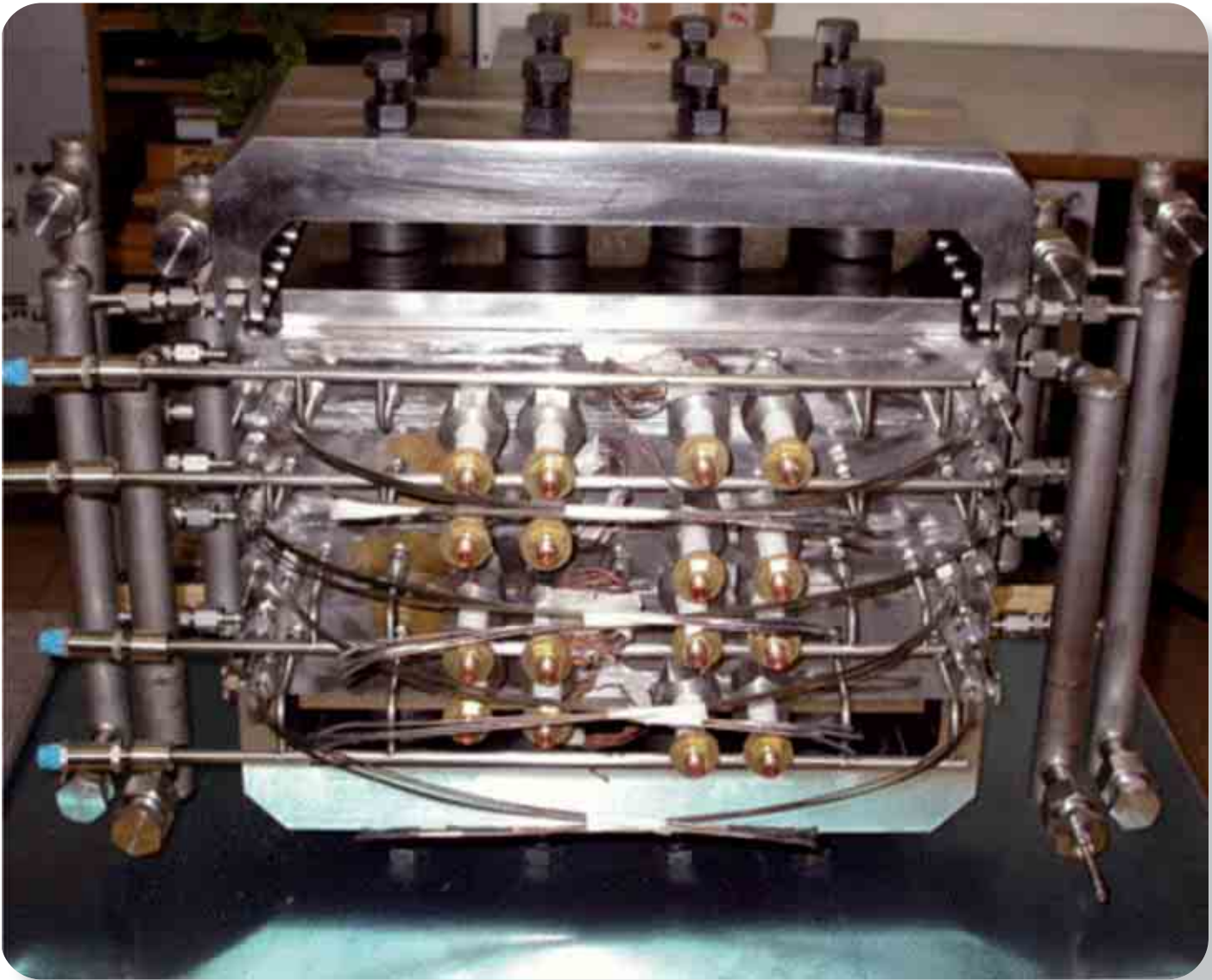
Sezione di prova di mantello triziogeno HEXCALIBER (HE-FUS 3 EXperimental CAssette of Lithium BERYllium Pebble Beds). Tritium breeding blanket test section of HEXCALIBER (HE-FUS 3 EXperimental CAssette of Lithium BERYllium Pebble Beds).
