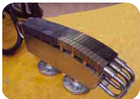
Prototipo del Inner Vertical Target - Prototype of the Inner Vertical Target (Ansaldo Ricerche and ENEA).
