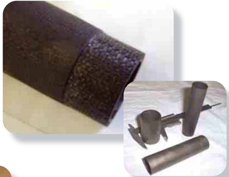
Tubo impermeabile a doppia parete in SiC: monolitico/composito. Double wall SiC non-permeable tube: monolithic/composite.
