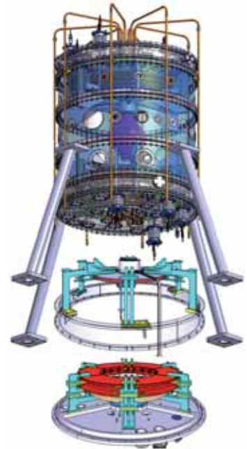
Fig. 1.37 – CAD model of MULTI-PINCH, showing the disassembling of the cathode group from below
