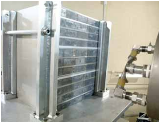
Fig. 3.23 – HCLL-TBM mockup in front of the FNG target
