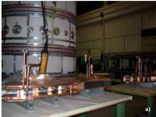
Fig. 1.38 – a) Modules of the final annular anode of MULTI-PINCH; b) annular cathode with 54 tungsten filaments
