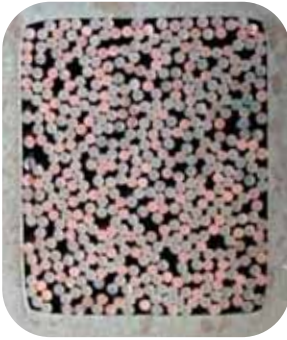
Fig. 4.3 – JT-60SA TF conductor sample cross section
