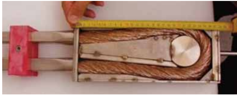
Fig. 4.4 – U-bent unjacketed JT-60SA TF conductor sample in the box substituting the bottom joint in the hairpin SULTAN sample
