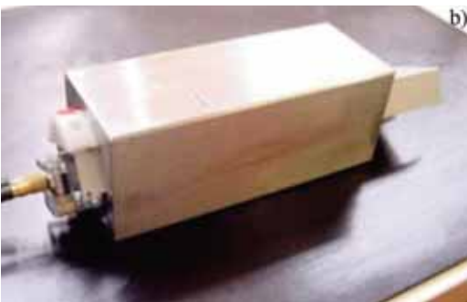
Fig. 3.12 – a) Jacket samples for reference blocks; b) miniaturised VRUT-3 TOFD boresonic device
