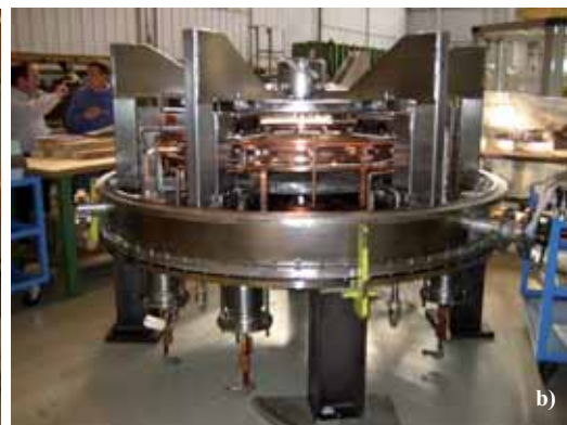
Fig. 1.39 – a) Anode group with nearby plasma shaping coils; b) cathode group
