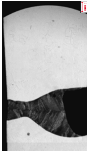
Fig. 3.17 – Typical macrosection of hybrid weld root pass
