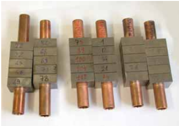
Fig. 3.1 – Tungsten monoblock samples manufactured by HRP
