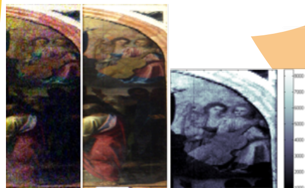
Fig. 2.42 - Comparison among RGB image obtained from raw data (left), RGB data from the whole visible spectrum (centre), IR image (right).
