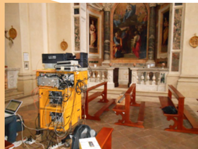
Fig. 2.37 - RGB-ITR laser-radar system assembled in a tower configuration during the field campaign by Santa Caterina della Rosa dei Funari Church (May 2013).
