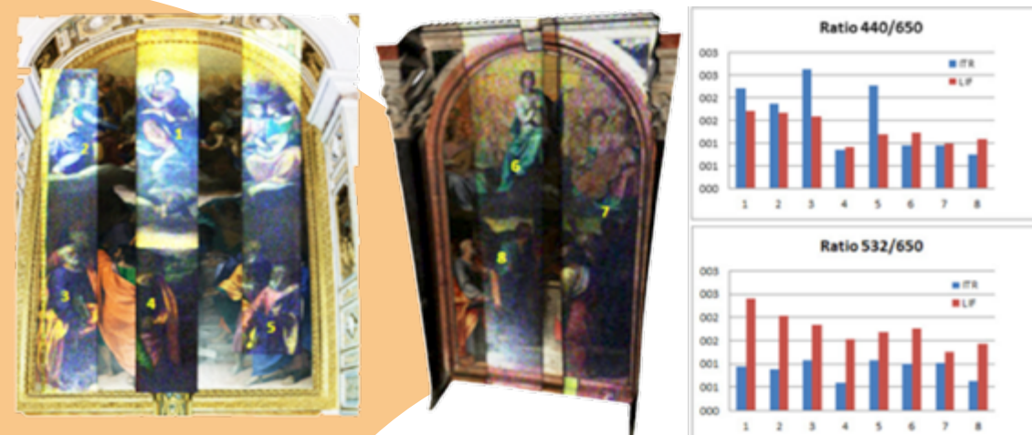
Fig. 2.41 - Overlap of reflectance images with RGB-ITR 3D color models: Bandini chapel (left), Solano chapel (center). Yellow numbers mark pixels where data reported on the right were collected representing the ratios from reflectance spectra recorded by the LIF scanning system at the working wavelengths (B = 440nm, G = 532nm, R=650nm) in comparison with B/R and G/R monochromatic ratios from the RGB-ITR at the same wavelengths.
