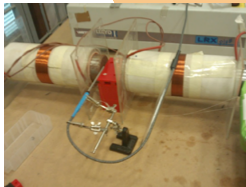
Fig. 4.16 - Test of the magnetic field sensor being performed by a electromagnet employed to provide a high and uniform field in its gap. The red box contains the sensor and allows its reliable and repeatable positioning.
