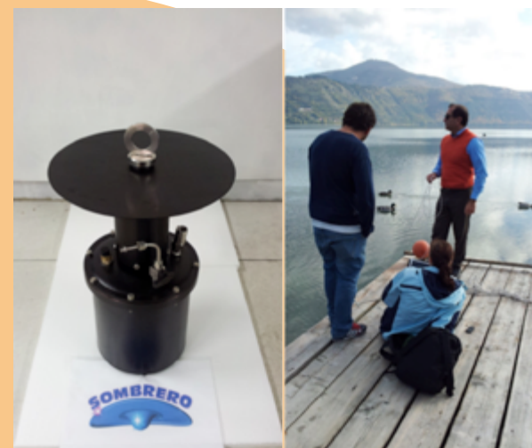
Fig. 2.32 - SOMBRERO spectrofluorometer (right) and during the test in the Albano Lake dipping it from a pier (left).
