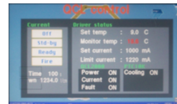
Fig. 2.6 - The TFT panel display implements a user friendly interface by the definition and use of softkeys (touch buttons).
