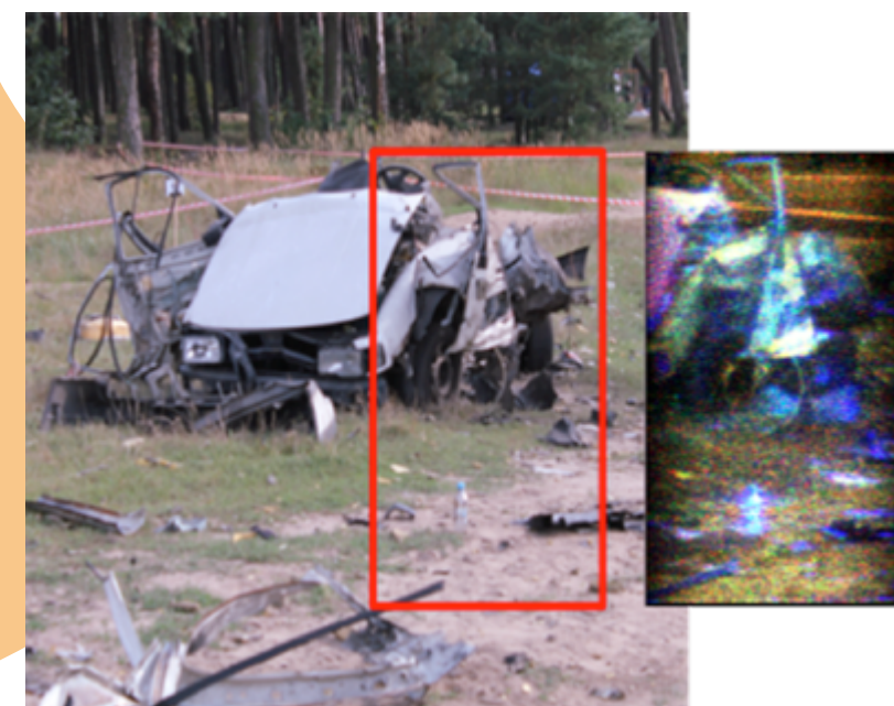
Fig. 2.14 - Conventional photo of the investigated area in Wroclaw (Poland) training on outdoor scenario (left side) and LIF image on a portion of the entire area restituted as three fluorescence band combination (right side).
