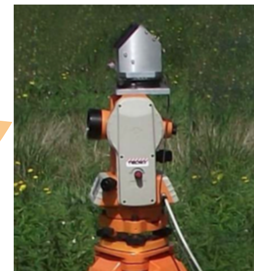
Fig. 5.7 - First ENEA electronic solar compass (prototype No 1) mounted on a theodolite.
