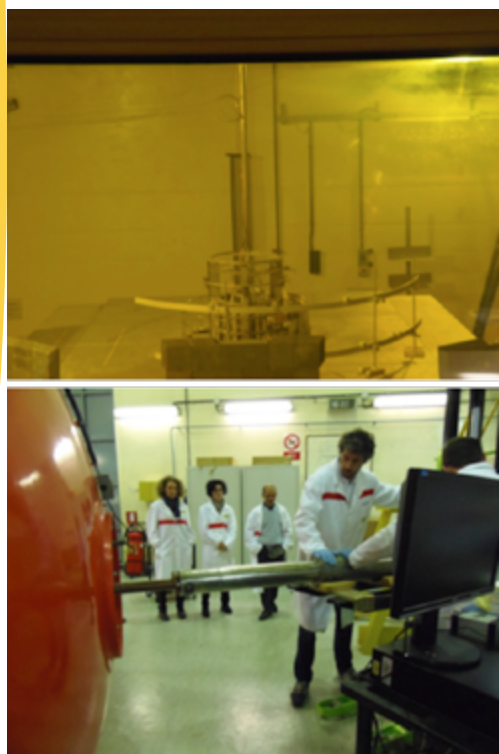
Fig. 2.48 - Top: piezo-motor test assembly on the CALLIOPE Facility. Bottom: insertion of the tested components in the TAPIRO neutron channel
