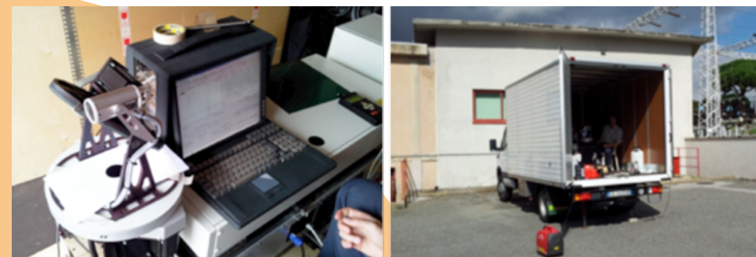
Fig. 2.8 - The lidar/DIAL (left) inside a van (right) during its test at the ENEA research center of Frascati. It was operated with a portable power supply (red box in front of the van).
