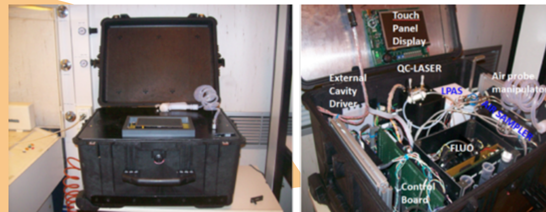
Fig. 2.5 - The complete CUSTOM sensor. The complete assembly in a portable case (Left). Open case, the LPAS and FLUO sensors are allocated inside (right).
