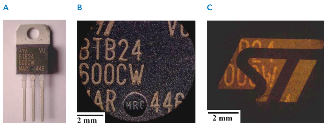
Figure 7: (a) Standard transistor with plastic packaging covered by a LiF film and exposed through a metallic mask to the EUV radiation from the DPP, as observed when illuminated with natural light. The treated area is observed by a microscope at low magnification (b) with white light illumination and (c) in fluorescence mode.
