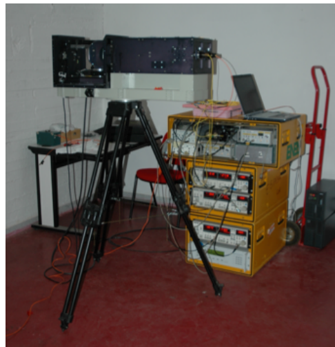
Figure 13 - Photo of the non-invasive RGB-ITR system used for high-resolution, high-accuracy 3D color imaging. The black box is the optical head hosting the launching and receiving optics along with the motors for the horizontal and vertical scanning. The yellow casing, instead, contains the electronic modules (lock-in amplifiers, motor controller, etc.) and the three AM laser sources whose light travels by optical fibers. A laptop is used for the remote operating of the RGB-ITR and for the analysis of the acquired data.
