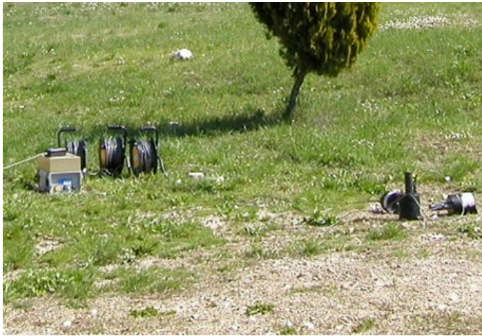
Figure 18. Site recording of ambient noise obtained by a Kinemetrics data acquisition system consisting of one K2 Digital Recorder connected to three SS1 velocity transducers, one for each component (N-S, W-E, Up) of the ground motion (left). Example of elaboration by the Nakamura's technique: plot of the Fourier spectra of the 3 components of ambient noise North-South, West-East and Up-Down (right-up); average spectral ratio of the Horizontal vs. Vertical components showing in this case a resonance frequency of the site at 1.8 Hz (right-down).
