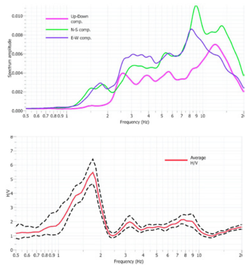
Figure 18. Site recording of ambient noise obtained by a Kinemetrics data acquisition system consisting of one K2 Digital Recorder connected to three SS1 velocity transducers, one for each component (N-S, W-E, Up) of the ground motion (left). Example of elaboration by the Nakamura's technique: plot of the Fourier spectra of the 3 components of ambient noise North-South, West-East and Up-Down (right-up); average spectral ratio of the Horizontal vs. Vertical components showing in this case a resonance frequency of the site at 1.8 Hz (right-down).
