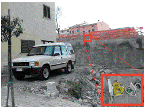
Figure 15. Structural monitoring of civil engineering works. Left: on-site monitoring of retaining walls by mobile laboratory; the inset shows the patch-panel with optical connectors to access the FBG sensors embedded in the concrete pouring. Right: aerial view of the monitored section of the roman ruins of the Mura Aureliane; the inset shows the ending of the optical fiber backbone used to collect the signal from the installed FBG sensors.
