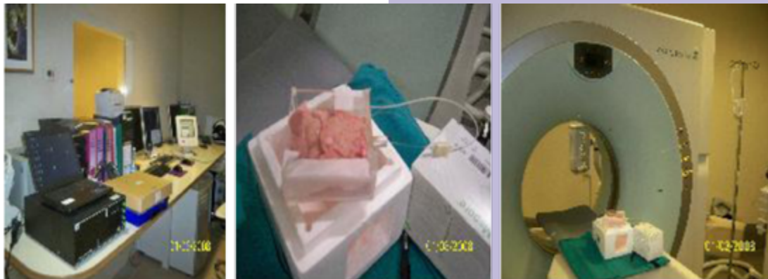
Fig. 16 - Use of fibre optic sensors for assessment of thermal effects due to the laser-pancreatic tissue interaction during LITT (Laser-induced interstitial thermotherapy): experimental research activity on ex-vivo porcine pancreas aimed to human surgery application.
