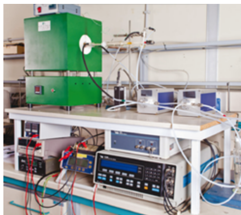
Fig. 43: Experimental methanation reactor.
