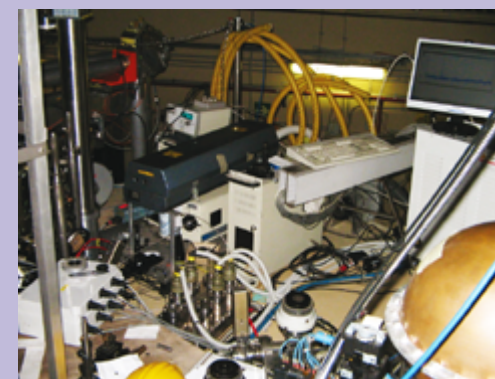
Fig. 39 - LIBS apparatus installed at the ENEA Fusion facility FTU. In detail, the apparatus and the optical window.
