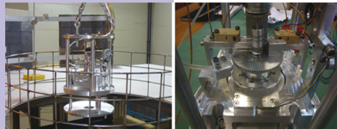
Fig. 37 - Left: piezo-motor test assembly on Calliope Facility. Right: detail of piezo-motor test assembly.
