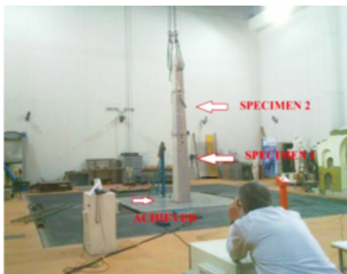
Fig. 20 - Model Lateran Obelisk placed on the shaking table
