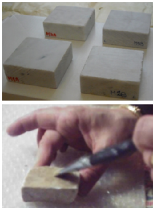
Fig. 32 - White and grey Carrara samples (top) and application of solutions by brushing (bottom).
