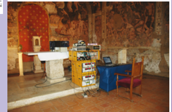
Fig. 24 - RGB-ITR system assembled in a tower configuration on a mobile platform. On the bottom: the first two boxes host a motion controller of the scanning motors and lock-in amplifiers for laser modulation and signals detection. Inside the next box: laser sources and detectors. On the top: the optical head with the scanning mirror. A laptop is used for the remote operating of RGB-ITR and for the analysis of the acquired data.
