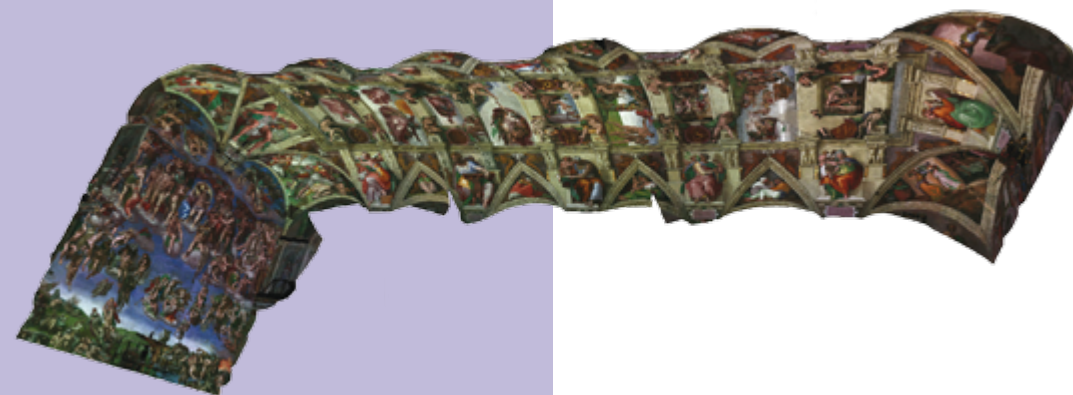
Fig. 25 - 3D color model of the Sistine Chapel after the application of the color calibration procedure: vault (40.5m x 13.5m x 20.5m) and Universal Judgment (13.5m x 18.5m) acquired by RGB-ITR system. This image is shown for scientific purposes only.
