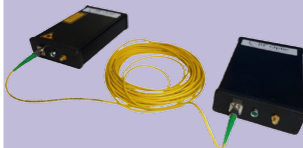
Fig. 29 - The modules for electrical to optical conversion of RF signals.
