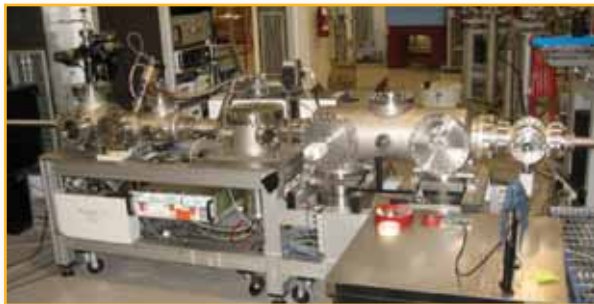
Figure 50 – Harmonic generation chamber realized at CEA. The laser enters from the left side and is optically matched to the undulator by two spherical mirrors located in the chamber on the right. The differential pumping ensures vacuum at 10^{-7} mbar in the electron beamline
