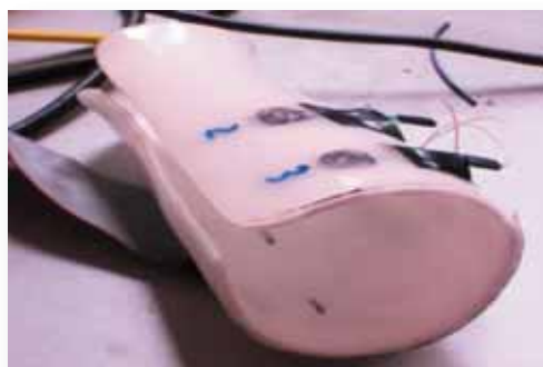
Figure 122 – Pressure sensors test prototype
