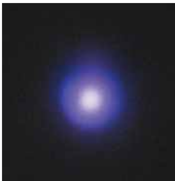
Figure 51 – Spot of the 266 nm radiation seed generated in gas as observed on a screen at about 15 m from the interaction point
