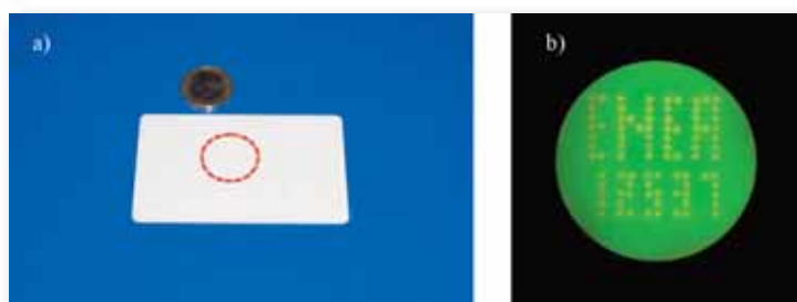
Figure 103 – a) Picture taken under natural light illumination of a standard plastic card (85 mm \times 54 mm) with an invisible mark within the dashed area written by the radiation emitted by EGERIA. b) Picture of the same dashed area shown in a), but with the pattern made visible by means of the compact and portable ENEA reading system prototype
