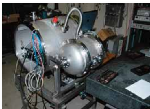
Figure 27 – RE-VUE during the operations of maintenance in the laboratory. The small cylinder hosts the laser, the scanning system and the receiving optics. The big cylinder contains the electronic modules
