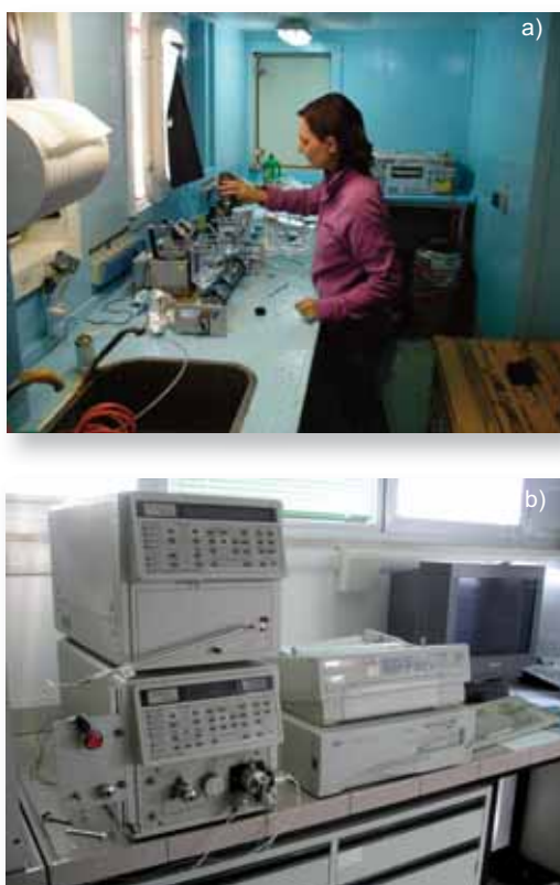
Figure 12 - TYR01 campaign: a) filtration ramp for phytoplankton sampling inside the Urania vessel, and b) HPLC equipment for marine pigment analysis
