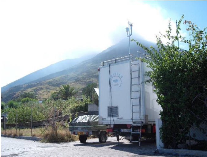
Figure 1 - The mobile lidar ATLAS at Stromboli, Italy. The laser has been aimed to analyze the volcanic plume.
