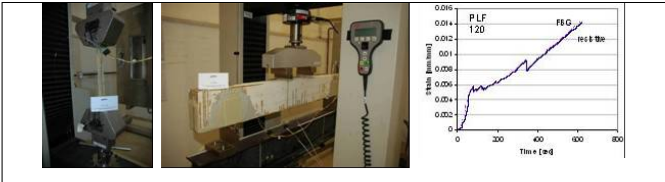
Fig.93. Textile laminated patch prototype (right). Small size beam reinforced by the developed smart textile (centre). Comparison of results from the sensor embedded in the smart textile with the results from a reference traditional sensor (left).
