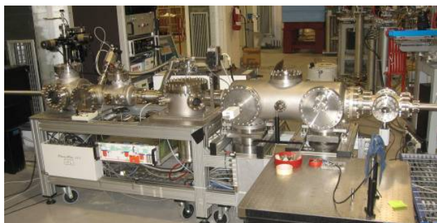
Figure 50. Harmonic generation chamber realized at CEA. The laser enters from the left side and is optically matched to the undulator by two spherical mirrors located in the chamber on the right. The differential pumping ensures vacuum at 10^{-7} mbar in the electron beamline.
