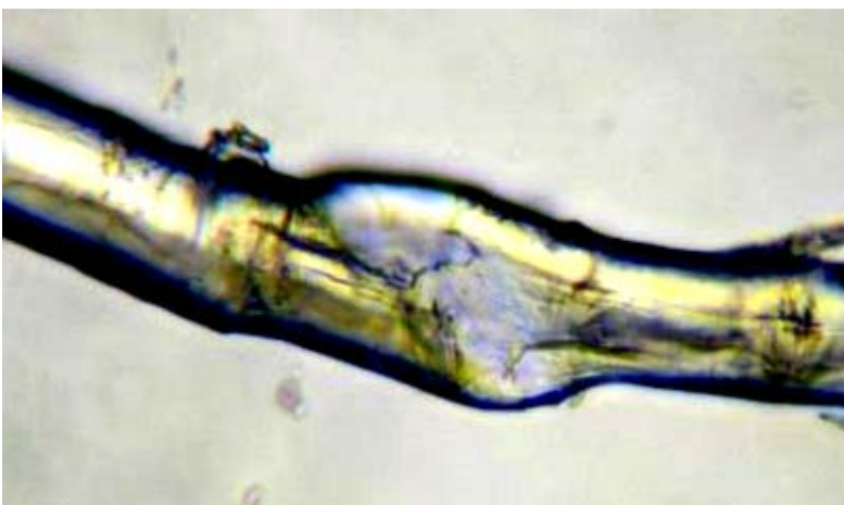
Figure 104 - Microscope view of a single fiber of linen colored after excimer laser irradiation at \lambda = 193 nm. The mechanical damage in the middle shows a colorless medulla, suggesting the color penetrates only the primary cell wall of the fiber, which is about 0.2 \mu\text{m} thick. The fiber has an average diameter of 20 \mu\text{m} .
