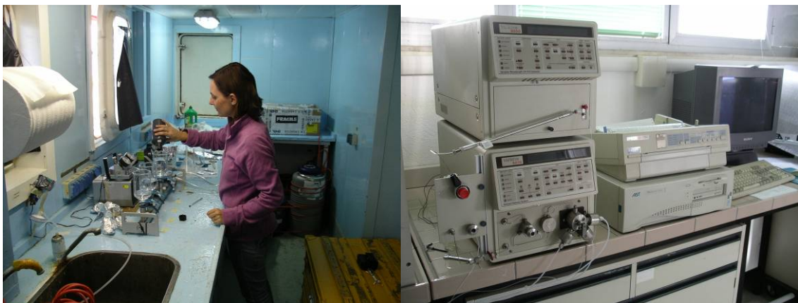
Figure 12 - TYR01 campaign: filtration ramp for phytoplankton sampling inside the Urania vessel (left) and HPLC equipment for marine pigment analysis (right).
