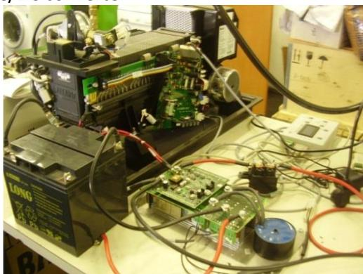
**Figura 7. Fuel Cell NEXA Ballard da 1.2 kW.**
