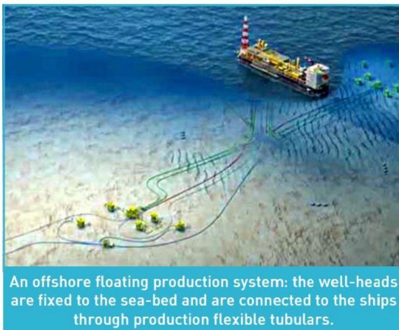
Figura 7 – An offshore floating production system
