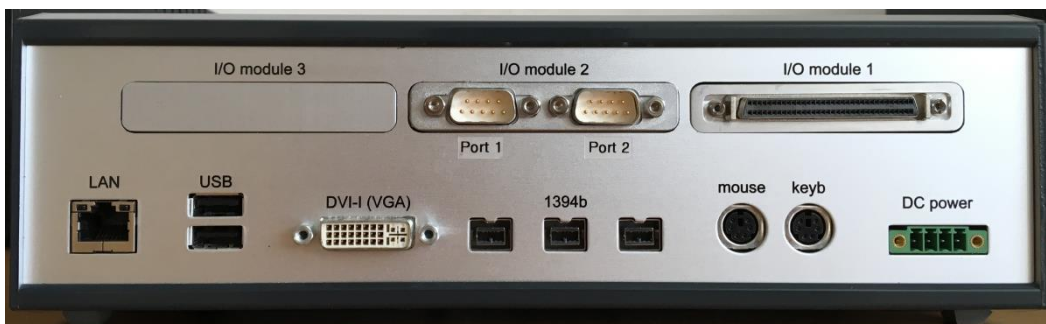
Figura 78: I/O di Speedgoat real-time target machine
