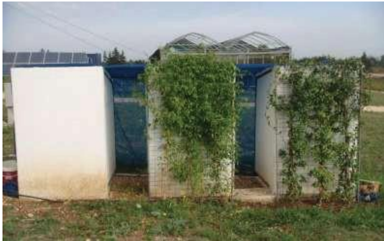
Figure 1: The three walls at the experimental field of the University of Bari; the right wall is covered with Rhynchospermum jasminoides , the central wall with Pandorea jasminoides variegated and the left wall is the uncovered control
