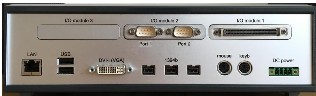
Figura 128: I/O di Speedgoat real-time target machine
