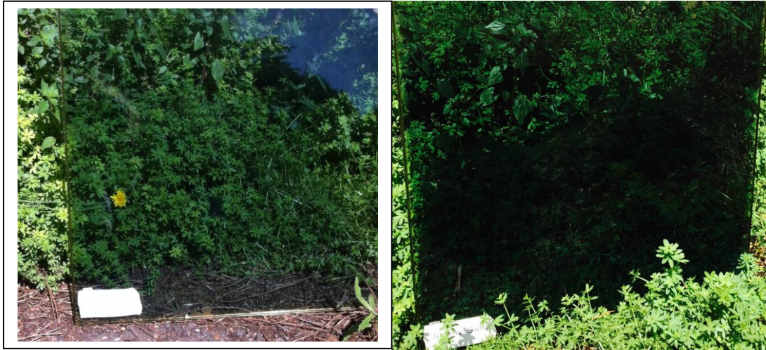
Fig. 1. Different states of TC glass, 400 x 400 mm sample under direct solar radiation.
