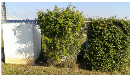
Figure 1. The three walls at the experimental field of the University of Bari; the right wall is covered with Rhyncospermum jasminoides , the central wall with Pandorea jasminoides variegated and the left wall is the uncovered control.
