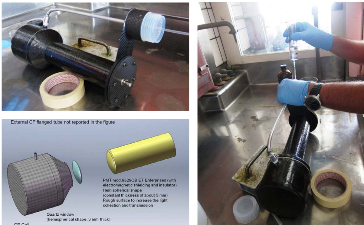
Fig. 3. Image and sketch of a C6D6 detector: in evidence, the main module, and the expansion system which prevents the formation of air bubbles inside the detector head and compensates thermal expansion [8].
