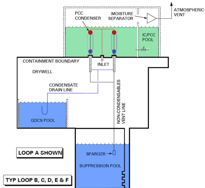
Figure 1: ESBWR Passive Containment Cooling System (redundancy degree not reported)
