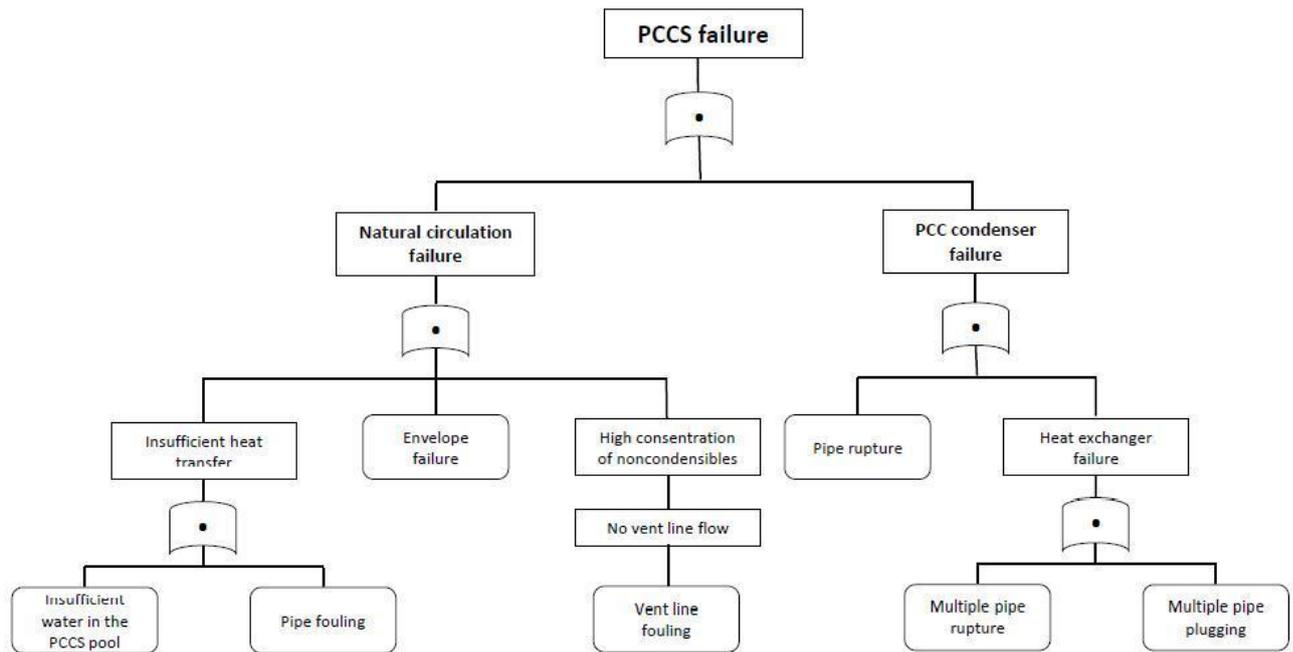
Figure 2: Fault tree for PCCS
