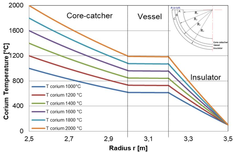
Figure 9: Radial temperature variation in the hemispherical bottom head for  $T(R_4) = 100\text{ °C}$ .
