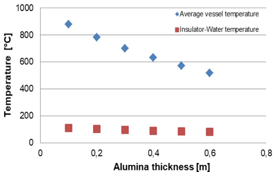
Figure 8: Temperature trend for different core-catcher thickness
