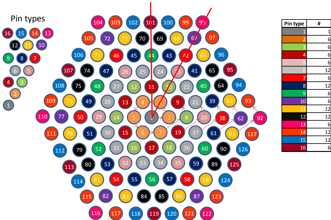
Figure A.1 Pins numbering and symmetry adopted by the ECCO cell code within the FA.
