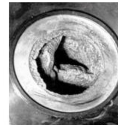
Slag deposit in the circuit during circulation pump tests
