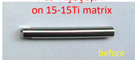
FeCrSi 0.4 \mu\text{m} PLD- \text{Al}_2\text{O}_3 1 \mu\text{m} on 15-15Ti matrix
