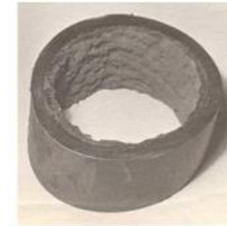
Slag in pipeline
