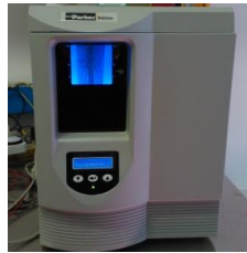
H-generator + mass flow controller for dosing c H2 in argon
