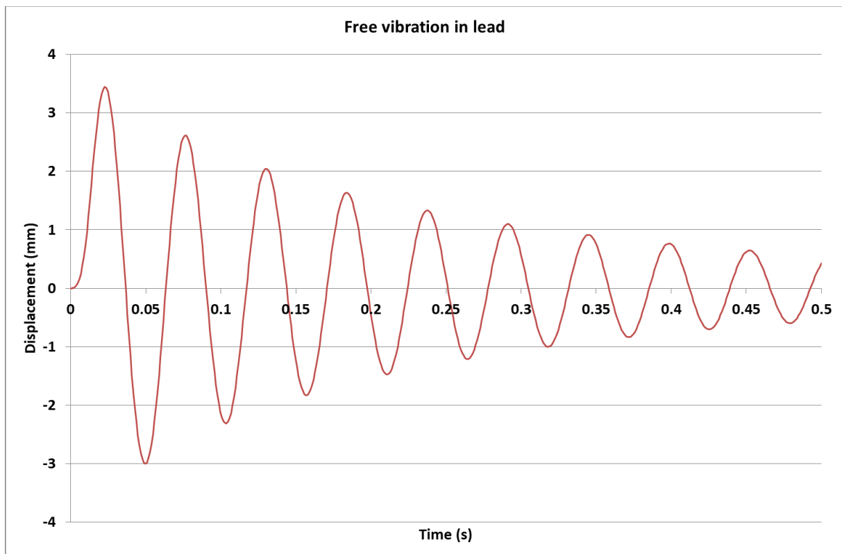
Figure 13. Pin displacement during free vibration in lead.
