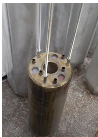
Figure 2.3 View of the ALFRED test section (left) and its positioning in the central hexagonal channel (right).
