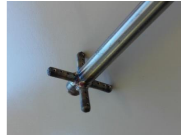
multi-holes gas injector in the raiser column (5 m long)
