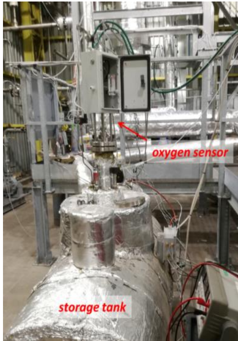
Calibration & Test at High Pressure in Pb storage tank
