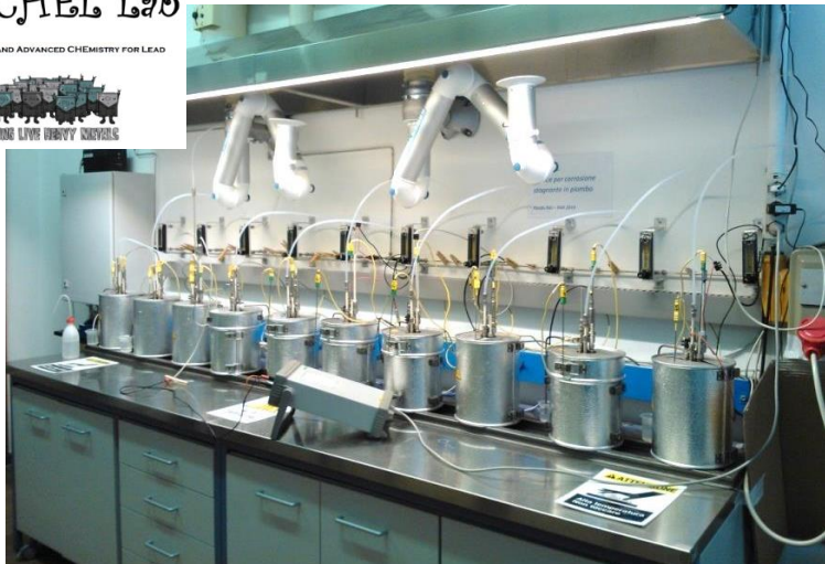
capsules for HLM chemistry & corrosion tests (750 g liquid Pb)
