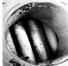
Slag deposit in heat exchanger
