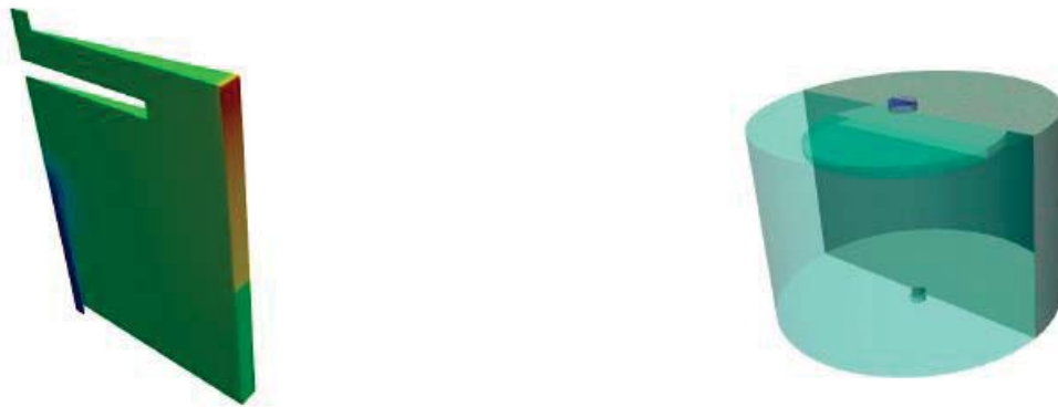
Fig. 4.9 - OpenFoam modelling for TALL-3D. The three-dimensional test section in Open Foam mesh (format in UNIV or MED).
