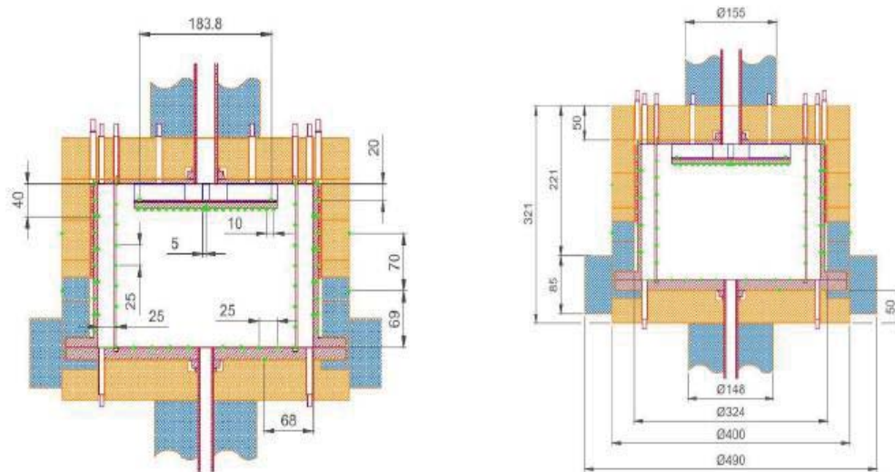
Fig. 4.8 - Modelling for TALL-3D. Geometry and dimensions.
