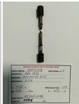
Fig.6 - Prova 550°C – 429 Mpa
