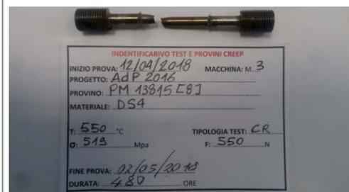
**Fig.3 - Prova 550°C – 519 Mpa**
