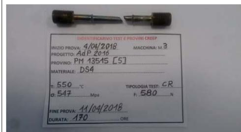
**Fig.2 - Prova 550°C – 547 Mpa**
