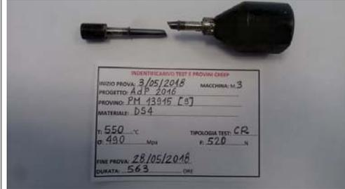
Fig.4 - Prova 550°C – 490 Mpa
