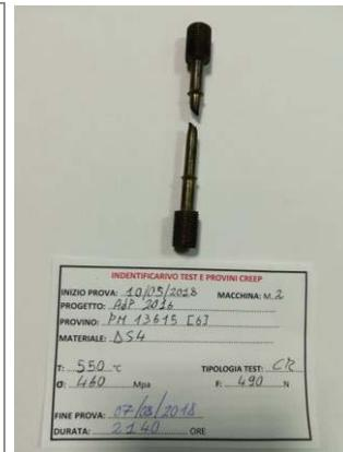
Fig.5 - Prova 550°C – 462 Mpa
