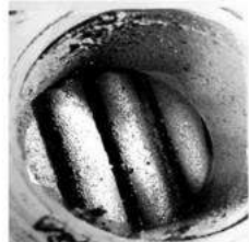
Slag deposit in heat exchanger
