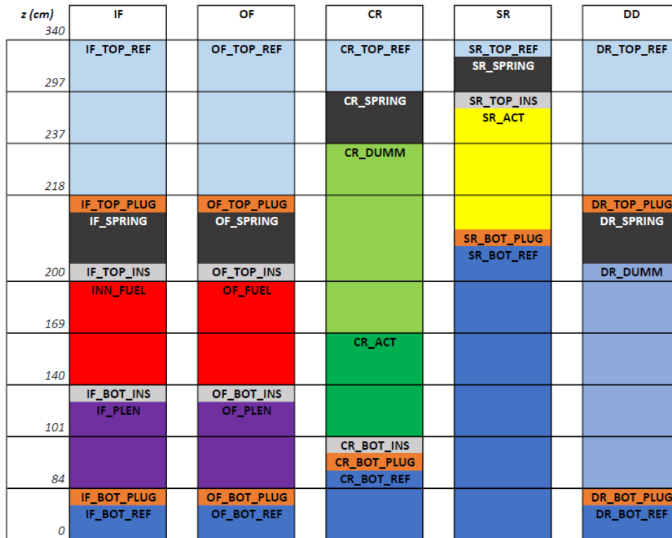
Fig. 5.4: core configuration with rod position adjusted to reach a condition closer to criticality.
