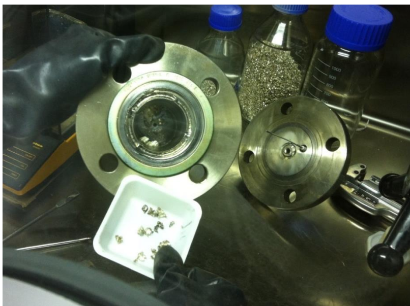
Figure 8: Lithium transferred in the bowl and remained in the sampler (inside the glovebox)
