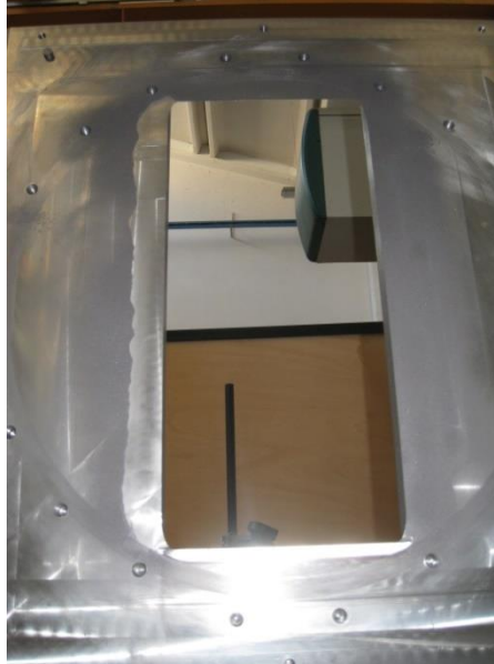
Fig. 14 Full size mockup of the supporting frame for the backplate.
