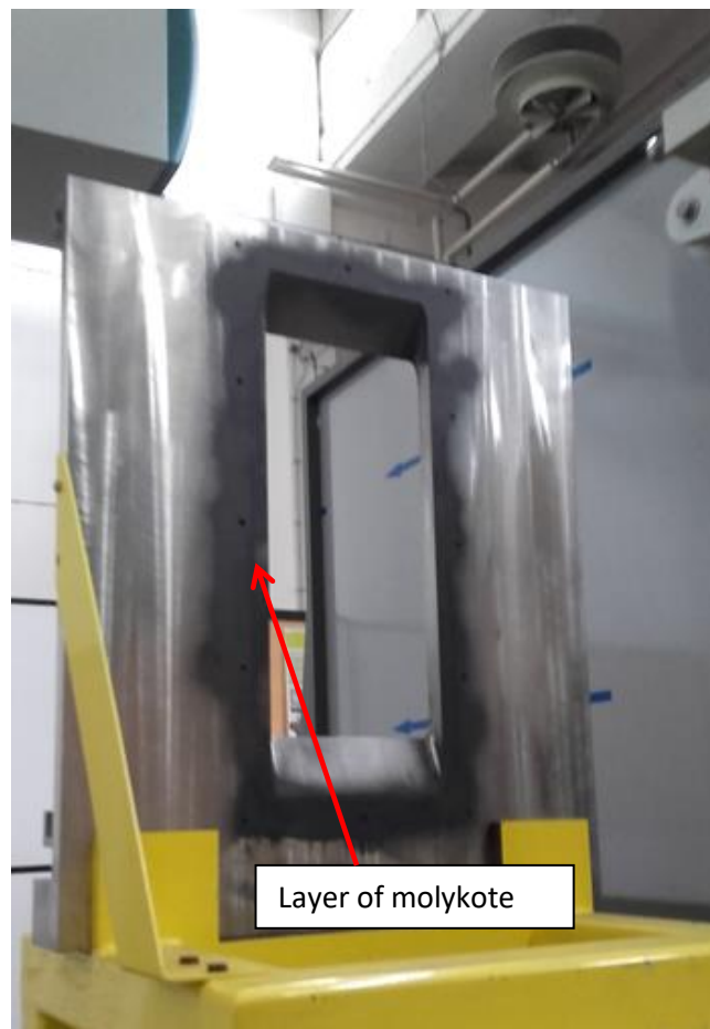
Fig. 16. Backplate support frame mockup sprayed with molykote
