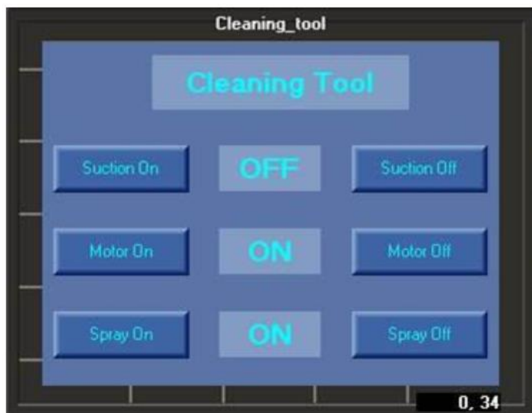
Fig. 12 New PLC GUI integrated in the exiting control system of the DRP facility
