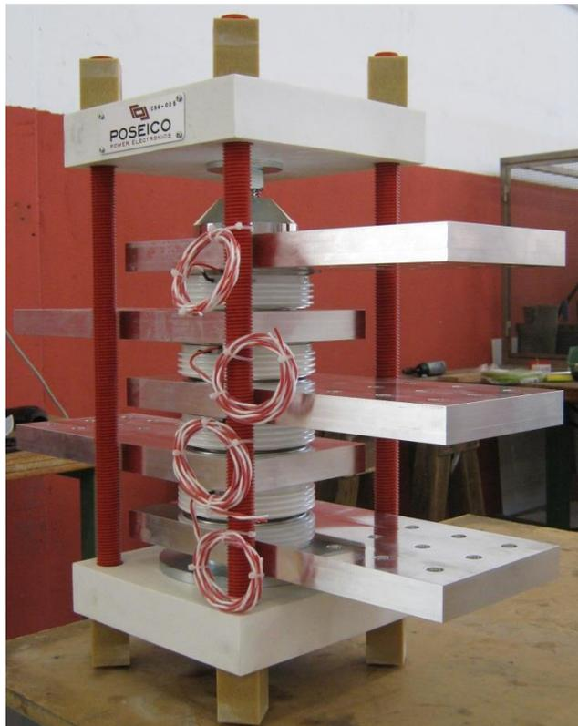
Figura 7 – Crowbar power assembly CS2/CS3
