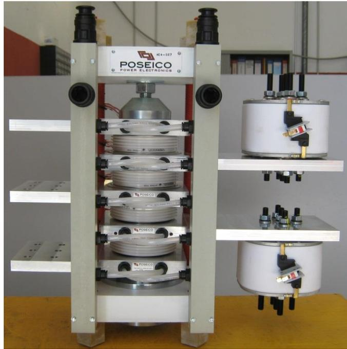
Figura 6 – Vista posteriore del CS2 power assembly.
