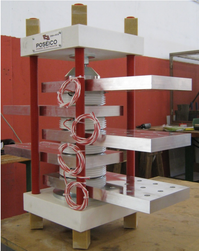
Figura 8 – Crowbar power assembly EF1/EF6
