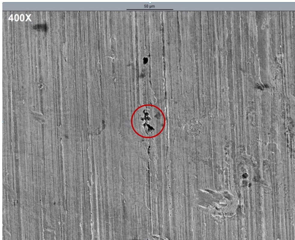
Figure 55: SEM image of specimen #29 surface (secondary electrons) at magnitude 400X. Scale bar above the image.
