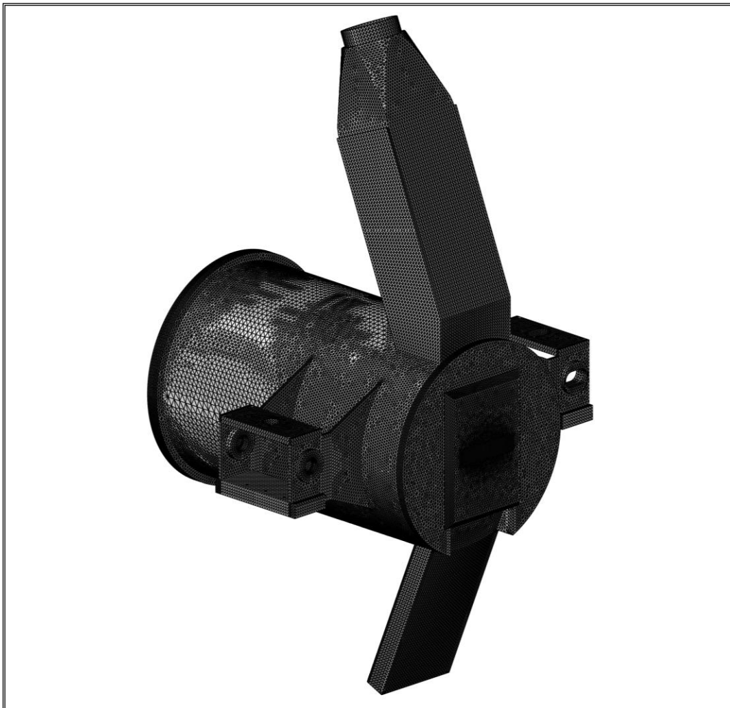
Figure 5. FEM model - Target Assembly.
