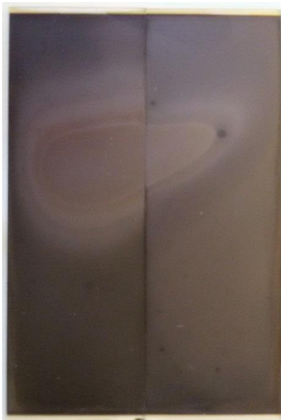
KN636: config. Originale (niente) T_{\text{piattello}}=545 , T_{\text{forno}}=585 t_{\text{dwell}}=60' \Phi_{\text{carrier}}=1 l/min; \Phi_{\text{N}_2}=0.5 l/min T_{\text{S}_2}=190^\circ\text{C}
