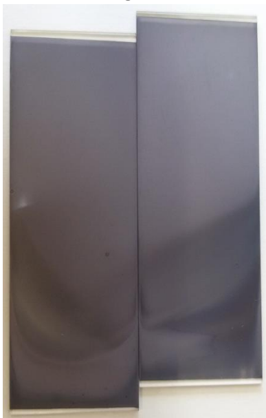
KN641: niente S T_{\text{forno}}=585 , T_{\text{piattello}}=545 , t_{\text{dwell}}=30' \Phi_{\text{carrier}}=1 l/min; \Phi_{\text{N}_2}=0.5 l/min T_{\text{S}_2}=190^\circ\text{C} – senza crogiuolo
