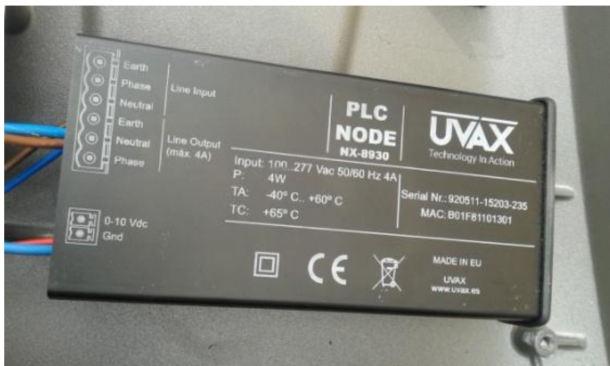
Figura 19 PLC NODE UVAX
