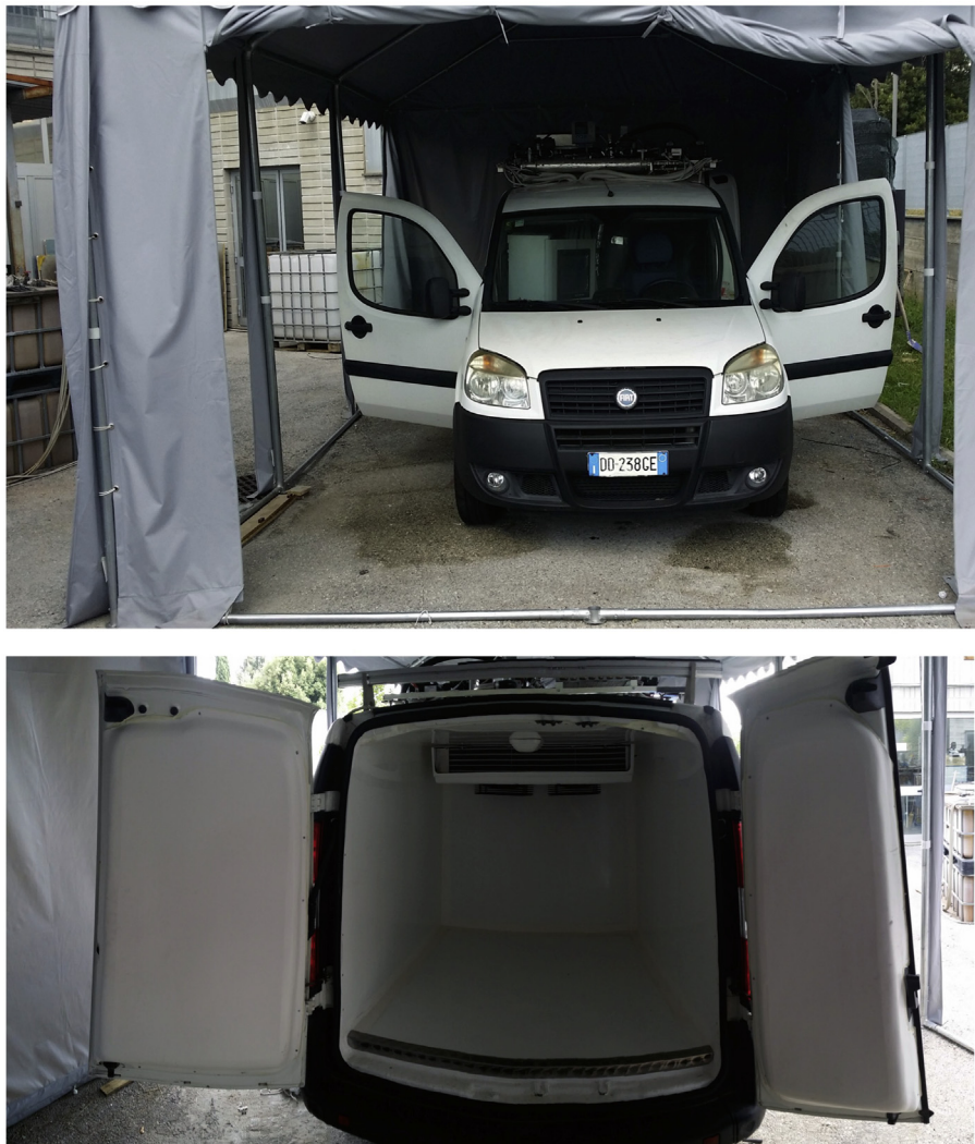
Fig. 12. Picture views of the vehicle with the assembled Metal Hydride Cooling System prototype (top). In the bottom an image of the insulated refrigerated van with its internal heat exchanger is shown.
