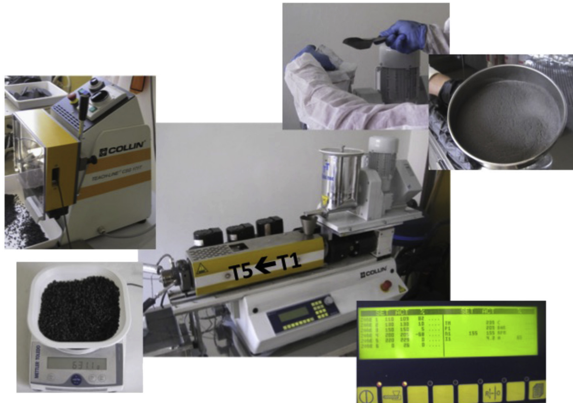
Fig. 5. Twin screw Collin ZK25TSCR15 extruder utilised to obtain the metal hydride - polymer composite. In the right up side the metal-matrix-filler blend obtained by ball milling is loaded into the dosing unit; the blend is extruded through the successive thermal zones: in the right bottom side the T1-T5 temperature settings are shown on the control panel; the extruded composite at the output is water down cooled and reduced in pellets by means of the in-line pelletizer (left side).
