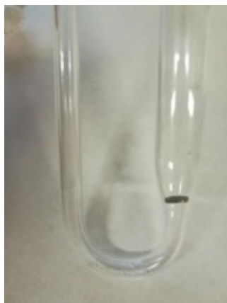
Figure 5. NiCo powders are compacted into a pellet (d=8mm, h=1mm) and placed in the quartz reactor. Reactive gases flow through the disc.
