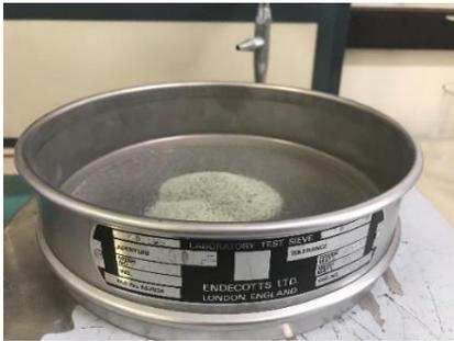
**Figura 27. Setaccio INOX ISO – 565, diametro 250  $\mu\text{m}$**
